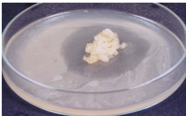
Figure 4 An example for the agar plate method for the evaluation of antibacterial activity of one of the gels. [Color figure can be viewed in the online issue, which is available at wileyonlinelibrary.com .]
